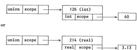
As with the primitive modes, the run time representation of a structure and reference to a structure are the same, i.e. The initial reference is suppressed as an optimization. The same arguments apply to rows and unions as well.
