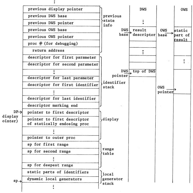
The range stack frame consists of 5 parts:
